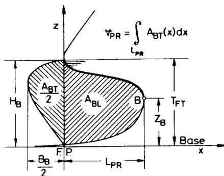
$$C_{ABT} = \frac{A_{BT}}{A_{MS}} \quad \text{Cross-section Coefficient}$$
