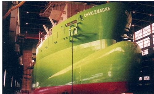
Example of a bulb of addition, with a knuckle in the intersection with the hull.
