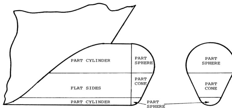
Bulb built from simplified conic shapes (Lamb, 1986 )
