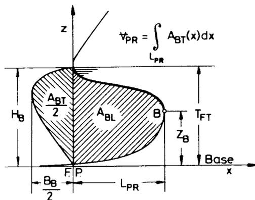
$$C_{BB} = \frac{B_B}{B} \quad \text{Breadth Coefficient}$$
