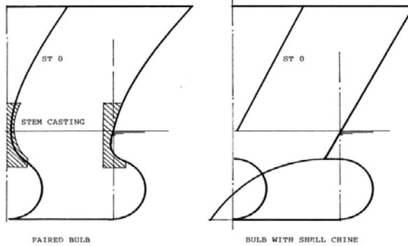
Bulb integrated and bulb of addition, with knuckle, avoiding a stem with a component in cast steel (Lamb, 1986 ).
