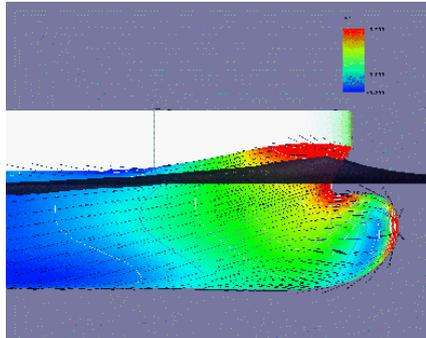
Combined representation of the wave profile, the distribution of the hydrodynamic pressure (colors) and of the flow lines
