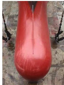
Examples of bulbs integrated in the hull.
