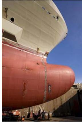
Examples of bulbs integrated in the hull shape.
