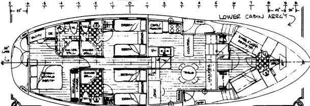
The 61' Aircraft Carrier (left) is a steel motoryacht that carries a float plane in addition to the usual small craft on the boat deck. She is laid out with the crew quarters for up to four forward, galley amidships, the saloon up behind the pilothouse, and three good sized staterooms with en suite heads aft for the owner and/or charter party.
